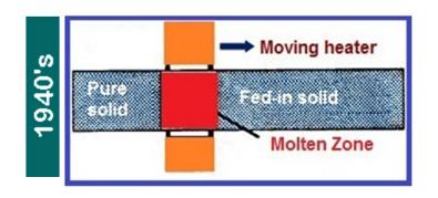
Zone refining – A metallurgical process to produce ultra pure Si
